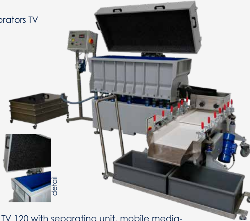
TV 120 with separating unit, mobile media-container and cascade for wastewater treatment
